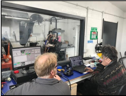
Engine cell control room
