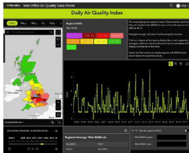
Figure 1. Example screenshot of data visualization tools used to interact with reanalysis data. This tool shows regionally averaged monthly maximum daily air quality index, with the map displaying values for April 2014 and the timeseries shown for the selected West Midlands area.
